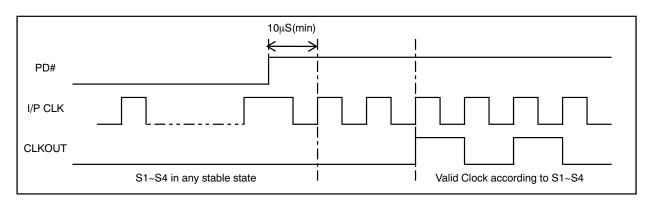
Note: Transition to new state will happen after a latency of up to 2 input clock cycles excluding the input cycle where the transition has occured.
