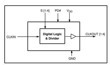
Figure 1. Block Diagram
