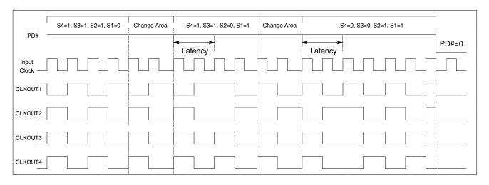
Note: Transition to new state will happen after a latency of one output clock cycle after completing the present output clock cycle Transition to new state will happen after a latency of up to 3 input clock cycles excluding the input cycle where the transition has occured.
