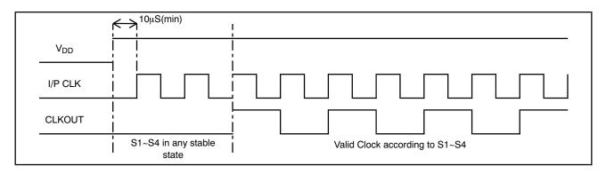
Note: Transition to new state will happen after a latency of up to 2 input clock cycles excluding the input cycle where the transition has occured.
